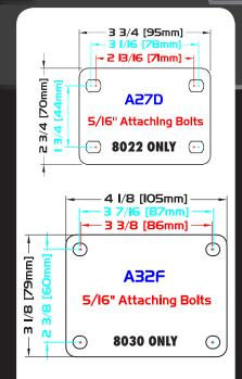
**STANDARD 8022 PLATE: A27D** D Plate Thickness: 3/32" F Plate Thickness: 5/32" **STANDARD 8030 PLATE: A32F**
